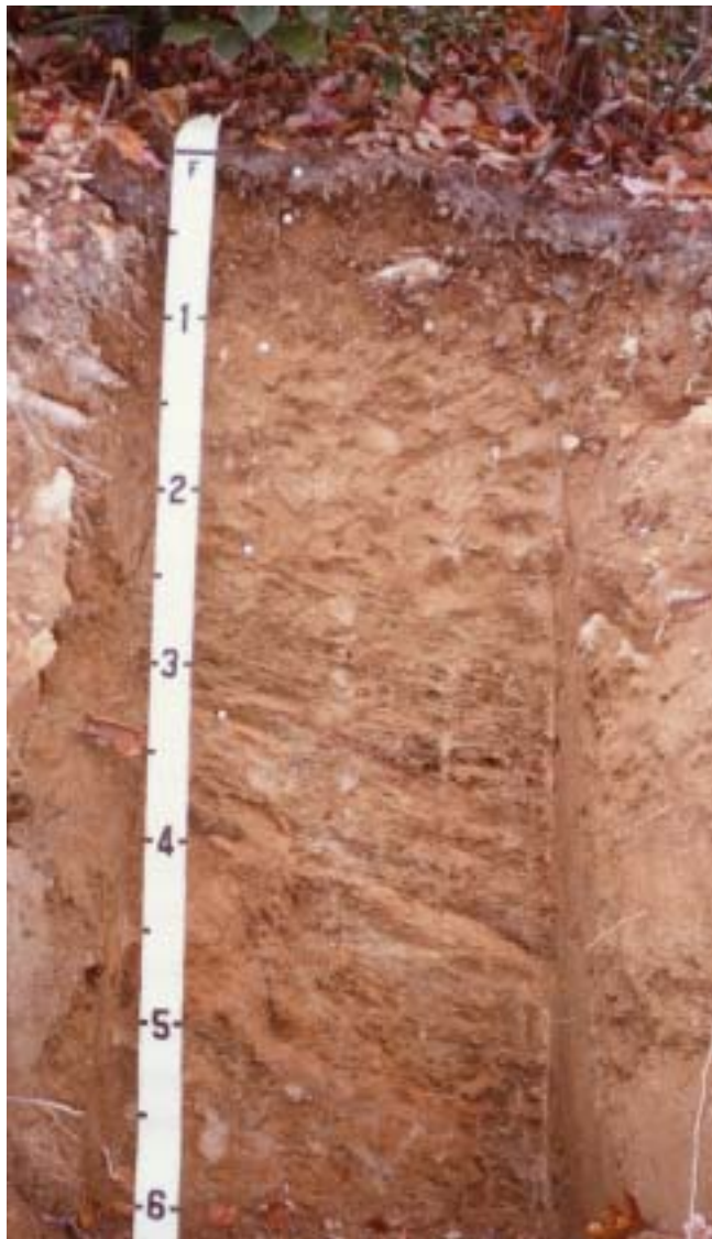
Figure 14.—Typical profile of Chandler fine sandy loam. Chandler soils have a high mica content in the subsoil and are very deep to soft bedrock. They occur on low and intermediate mountains predominantly in the southern half of Yancey County.
