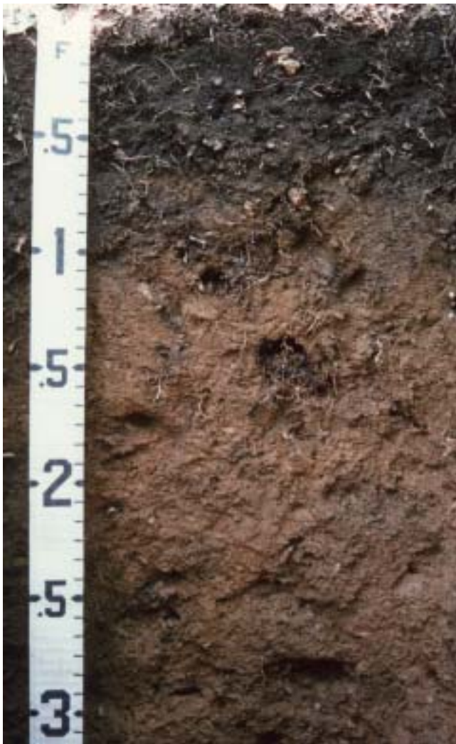
Figure 20.—Typical profile of Porters loam. Porters soils have thick, dark surface layers and are deep to hard bedrock. They occur on low and intermediate mountains throughout Yancey County.
