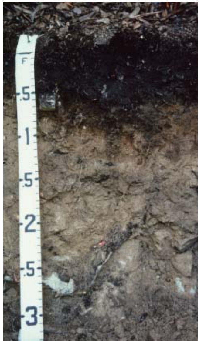
Figure 15.—Typical profile of Chestoa sandy loam. Chestoa soils have thick, dark surface layers and are moderately deep to hard bedrock. They occur on cool slopes of intermediate mountains in the Flattop area.
